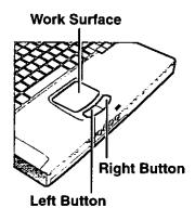
Use the touch pad to move the cursor on the display and perform normal computer operations.
